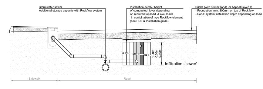
Cross section Line infiltration with parallel sewer Elements with different heights Scale 1:50
